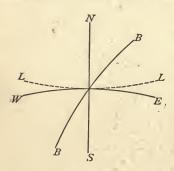
ing through it cuts from the spheroid a normal section. Of these the meridian section is the most important, and next is the prime vertical section, which is the normal section cut by a plane perpendicular to the meridian. These two sections are called principal normal sections because the properties of all other normal sec-
